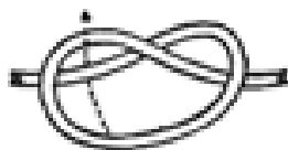
GUY-LINE HITCH can be lengthened or shortened as needed.
