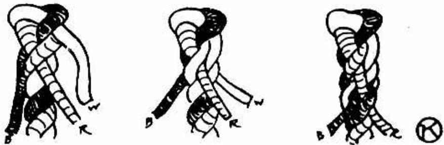
strand came out (C). Turn the rope over and tuck the third strand under the remaining strand of the standing part, going in where the first strand comes out (D).
