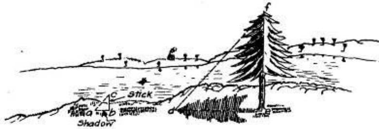
Stand your staff (b c) upright in the sun and carefully measure the length of its shadow (ab). Measure the length of the shadow of the tree. Multiply this by the length of the staff, and divide the result by the length of the staff's shadow. The answer will be the height of the tree.
